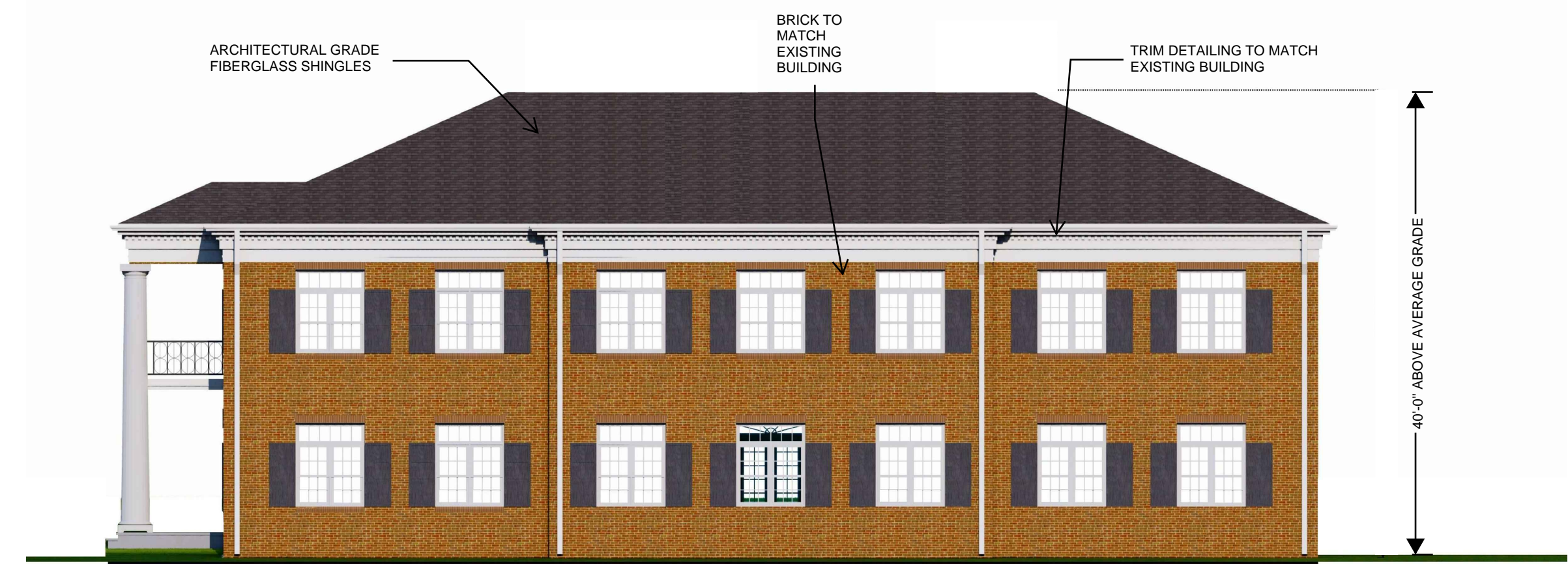
3 BUILDING ELEVATION - EAST
